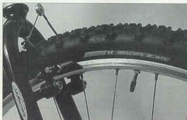
Dave Yates bikes in the South East, plugged in a pair of Joe Murray's triple butted Project Two forks. Triple butting means the tubing used in the forks' manufacture has three steps - thicker at the top, thinner at the bottom.
