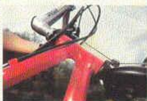
Immaculate fillet brazing is a Dave Yates trademark, not TIG welding that is common to most big production bikes.
