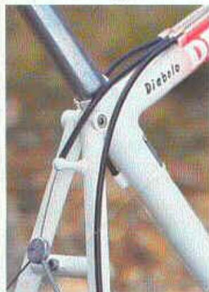
Touches like the neat single arm slotted cable guide are typical Dave Yates.
